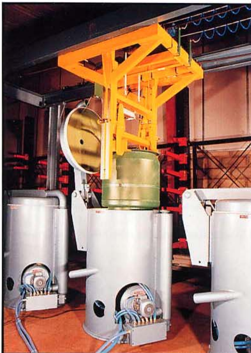
Centrifuge TA 60 Vx KCC2 integrated in an automatic line of spinning/drying of components after surface treatment.
