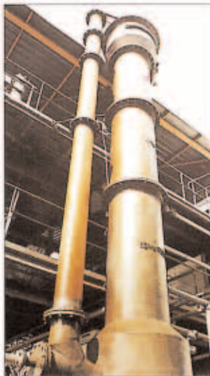
Colonne pulsée industrielle. Industrial pulsed column.
