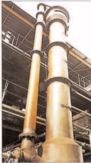
Colonne pulsée industrielle. Industrial pulsed column.
