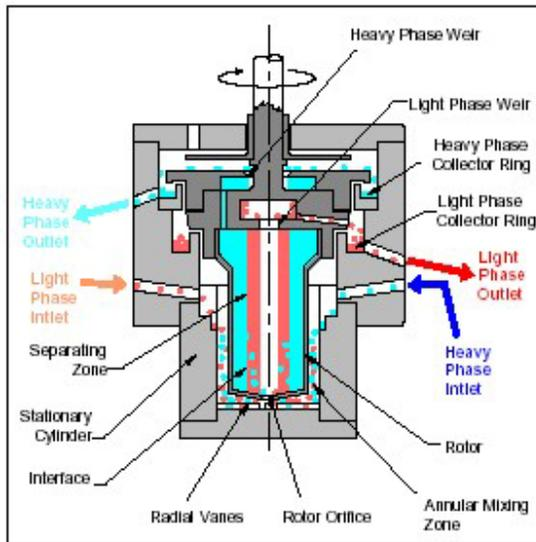
Fig. 1: Rousselet-Robatel annular centrifugal contactor
