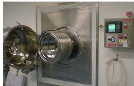
Figure 6: Horizontal basket centrifuge in a clean room with PLC control
