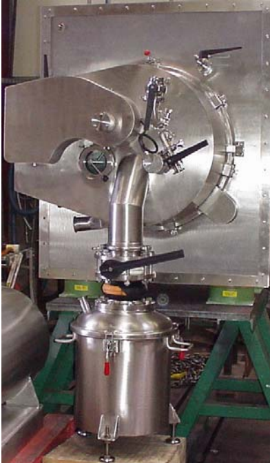
Figure 5: Pilot scale horizontal basket centrifuge with solids discharge into canister.
