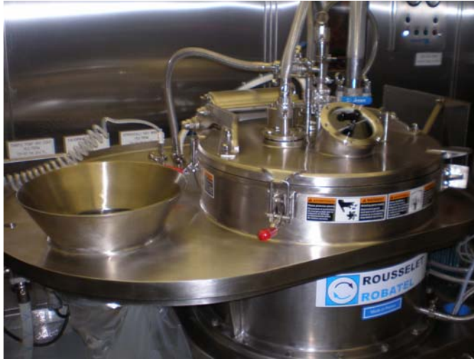
Figure 3: Pilot scale centrifuge with table for containment envelope, showing solids discharge hopper and low point drain [on left hand side of table]
