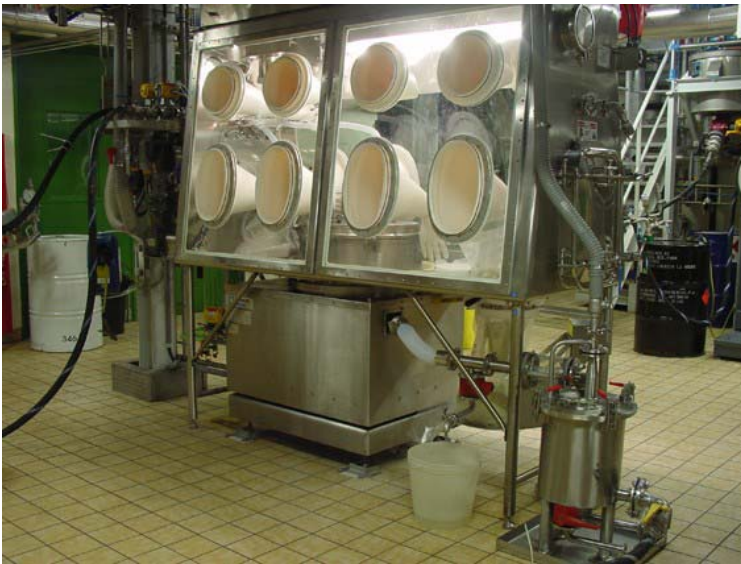
Figure 4: Pilot scale centrifuge installed in a glove box barrier-isolator.
