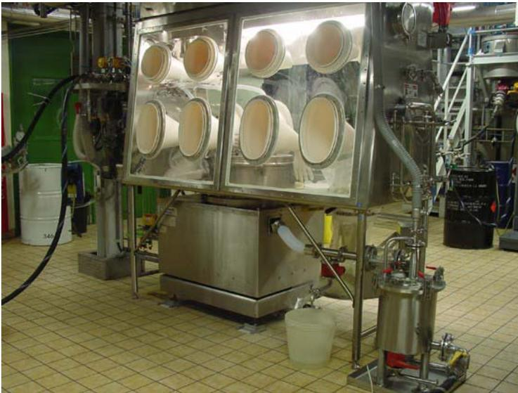
Figure 4: Pilot scale centrifuge installed in a glove box barrier-isolator.
