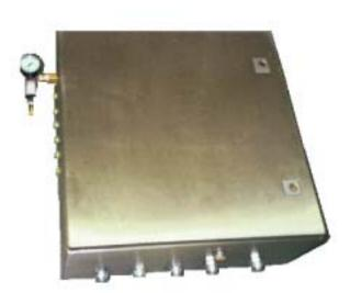
All machine mounted control wiring is pre-wired to a local junction box. This electrical enclosure is rated NEMA 4X and contains the terminal strip for the machine mounted low voltage electrical devices. In most cases, this is mounted to the side of the machine and machine wiring is done by ROBATEL. The customer would then connect the field wiring to the terminal blocks provided. The numbering on the terminal blocks is identical to the corresponding terminal block within the control cabinet.
