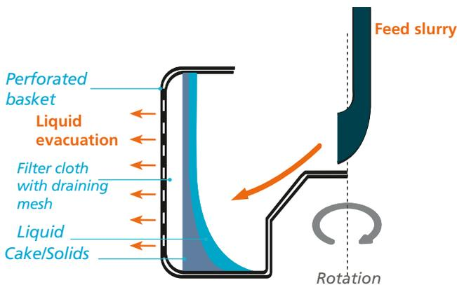
In this case the slurry can be fed into rotating basket.
