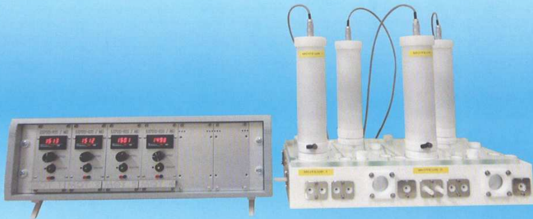
MD UX 1-4 : laboratory mixer settler, battery of 4 stages
